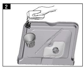
Remove the lower basket and then unscrew and remove the cap from the salt container. Place the end of the funnel(supplied) into the hole and introduce about 1.5kg of dishwasher salt. It is normal for a small amount of water to come out of the salt container. After filling the container, screw the cap tightly back clockwise.
