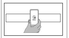
If you do not know the position of vour NFC antenna, slightly move the smartphone in a circular motion over the Smart Touch logo until the App confirms the connection. In order for the data transfer to be successful, it is essential TO KEEP SMARTPHONE ON DASHBOARD DURING THESE THE FEW SECONDS OF THE PROCEDURE: a message on the device will inform about the correct outcome of the operation and advise you when it is possible to move the smartphone awav.
