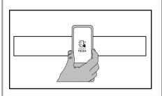
If you do not know the position of your NFC antenna. slightly move the smartphone in a circular motion over the Smart Touch logo until the App confirms the connection. In order for the data transfer to be successful, it is essential TO KEEP THE SMARTPHONE ON THE DASHBOARD DURING THESE THE FEW SECONDS OF THE PROCEDURE: a message on the device will inform about the correct outcome of the operation and advise you when it is possible to move the smartphone awav.
