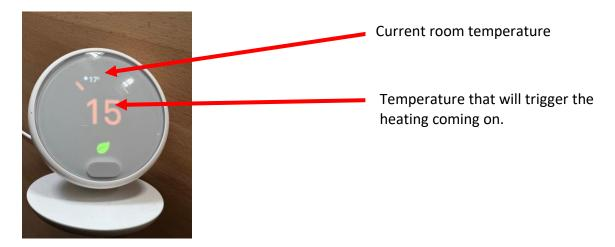
To increase the temperature of the lodge and allow the radiators to heat up you need to turn the outside ring of the thermostat clockwise. The large number in the middle will increase.
